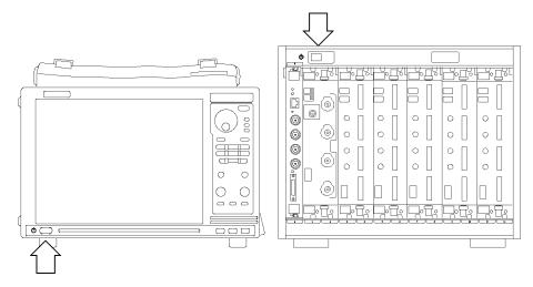
Figure 46: TLA7000 On/Standby switch locations
