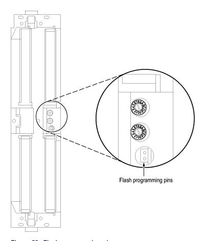
Figure 59: Flash programming pins
