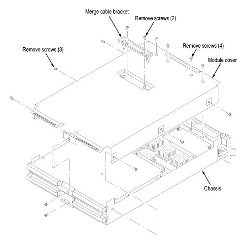
Figure 52: Removing the cover
