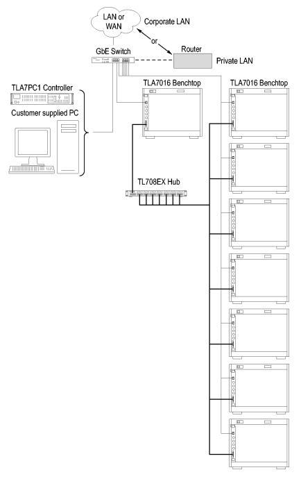
Figure 24: Expanded benchtop system with TL708EX Hub (up to 48 modules)
