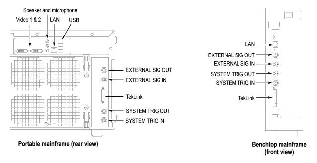
Figure 58: TLA7000 Series external connectors
