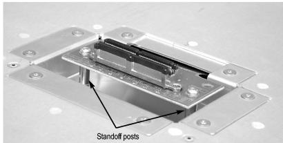
Figure 49: Removing the merger connector assembly from the module
