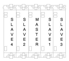
Figure 48: Location of modules in a merged system
