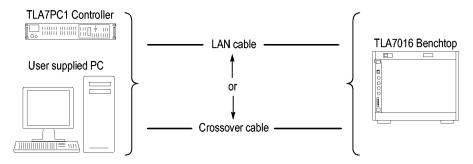
Figure 7: Benchtop mainframe setup (up to six modules)
