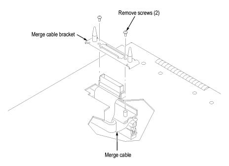
Figure 53: Feeding the merge cable through the cover
