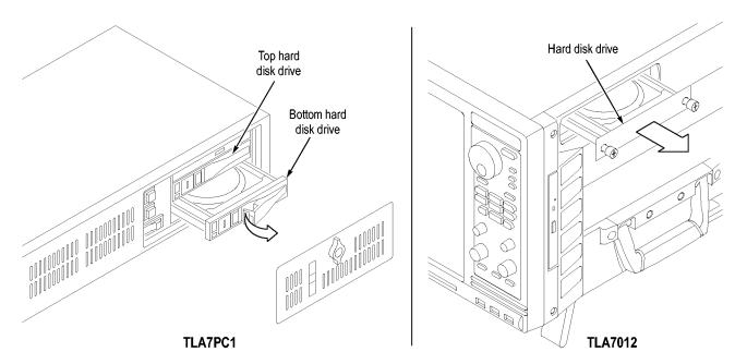
Figure 47: Accessing the replaceable hard disk drives
