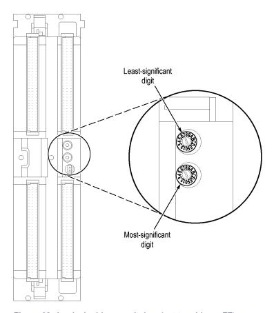
Figure 38: Logical address switches (set to address FF)
