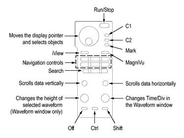
Figure 57: Portable mainframe front panel
