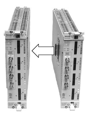
Figure 50: Connecting modules in a merged set
