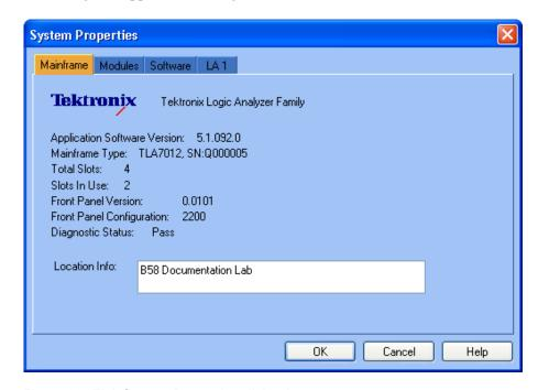
Figure 36: TLA System Properties dialog box
