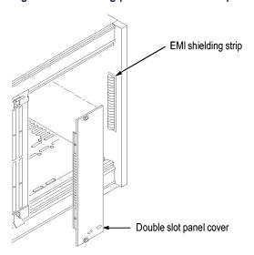
Figure 41: Installing panel covers on the benchtop mainframe
