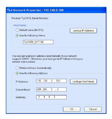
Figure 31: Make changes to the TLA network settings
