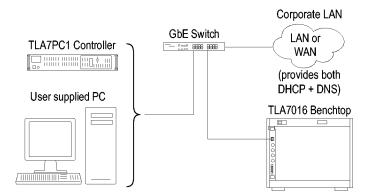
Figure 17: Benchtop mainframe corporate LAN setup (up to six modules)
