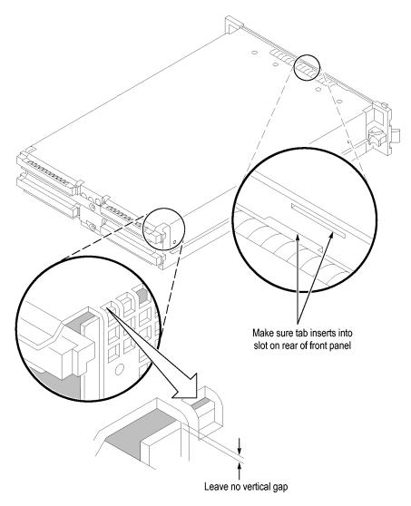
Figure 54: Seating the cover on the chassis
