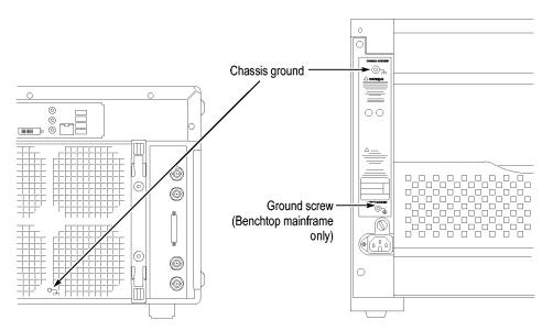
Figure 2: Location of the ground connection on the TLA7000 logic analyzers
