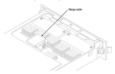
Figure 56: Positioning the merge cable before installing the cover
