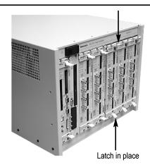
Figure 51: Installing the merged module set in the mainframe
