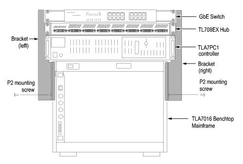
Figure 1: Bracket kit for the TL708EX Hub, TLA7PC1 controller and GbE switch installed on a TLA7016
