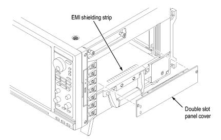
Figure 40: Installing panel covers on the portable mainframe
