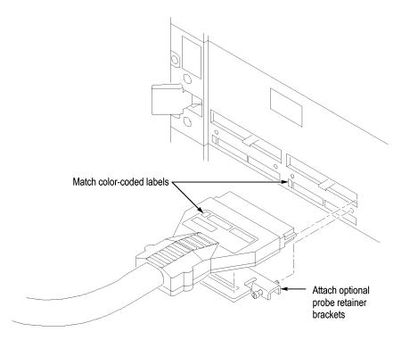
Figure 45: Connecting the P64xx logic analyzer probes to the TLA7Lx/Mx/Nx/Px/Qx logic analyzer modules
