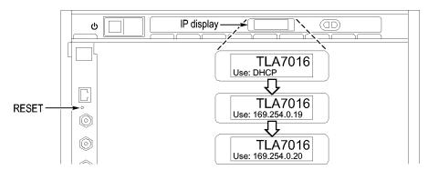
Figure 5: Setting the IP address
