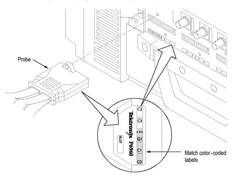
Figure 44: Connecting the P69xx logic analyzer probes to the TLA7Axx logic analyzer module
