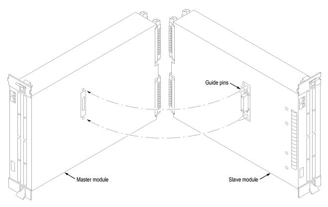
Figure 55: Lining up the two modules
